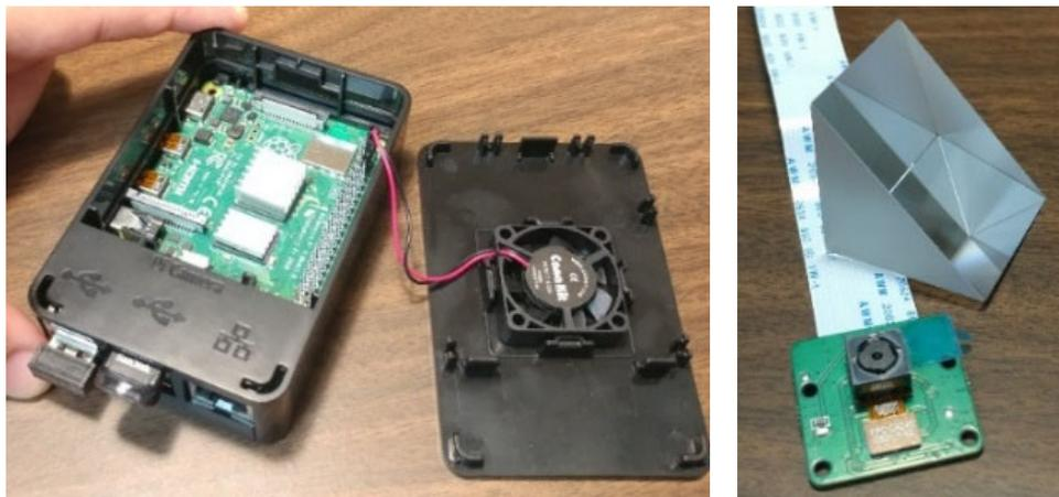
Figure 1 - Assembled Raspberry Pi 4, prism, and autofocus camera
